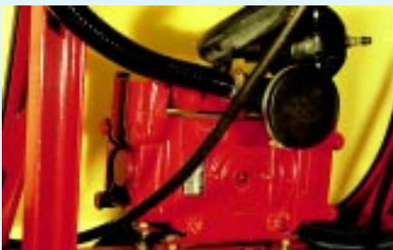
321/7.0 with pressure and suction damper
